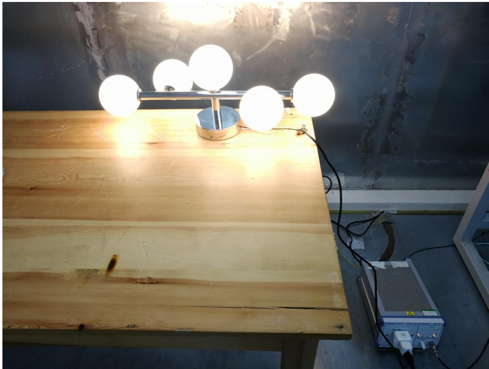
Photo of Power Line Conducted Measurement
