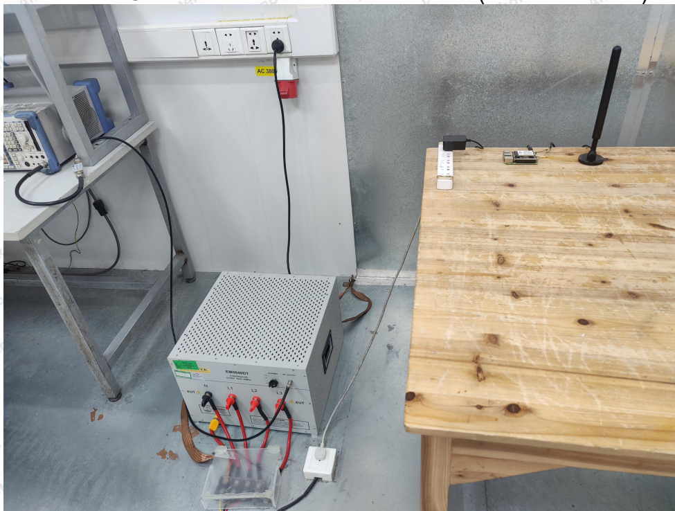
Photo of Conducted Emission Measurement (Sucker antenna)
