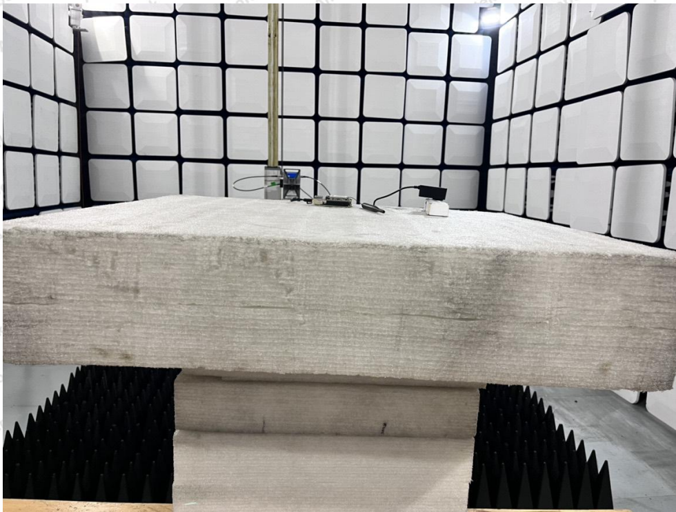
Photo of Radiation Emission Test (Sucker antenna)
