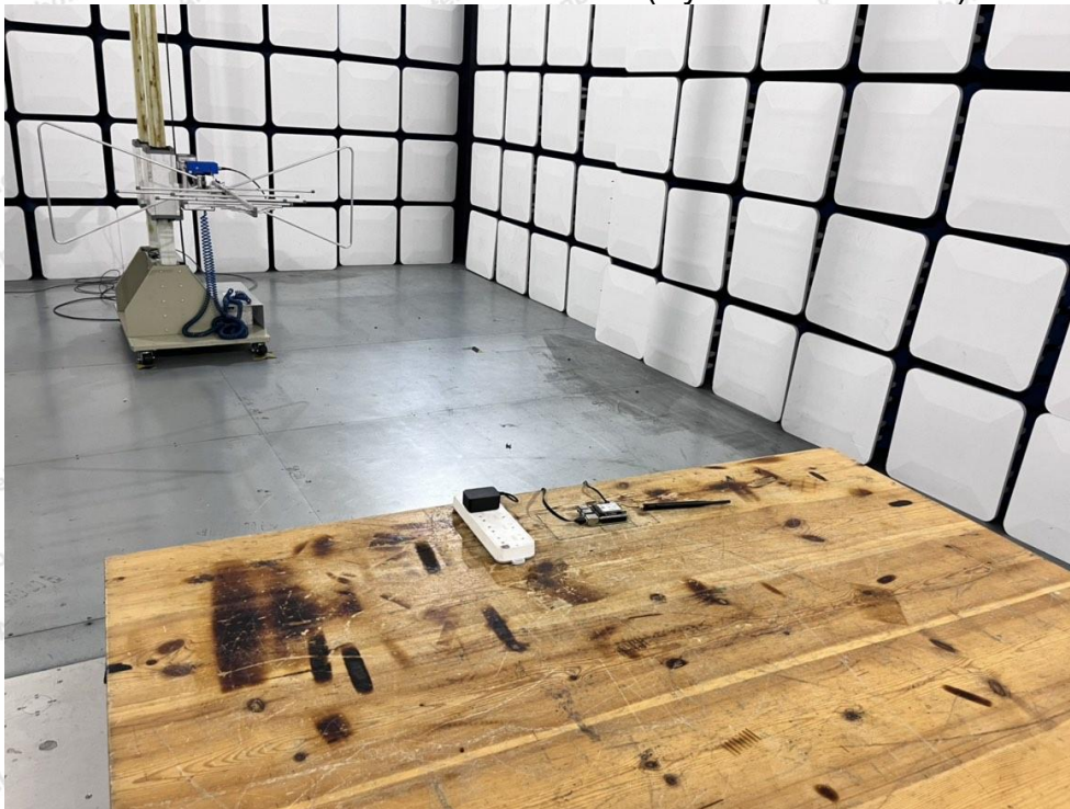
Photo of Radiation Emission Test (Cylindrical antenna)
