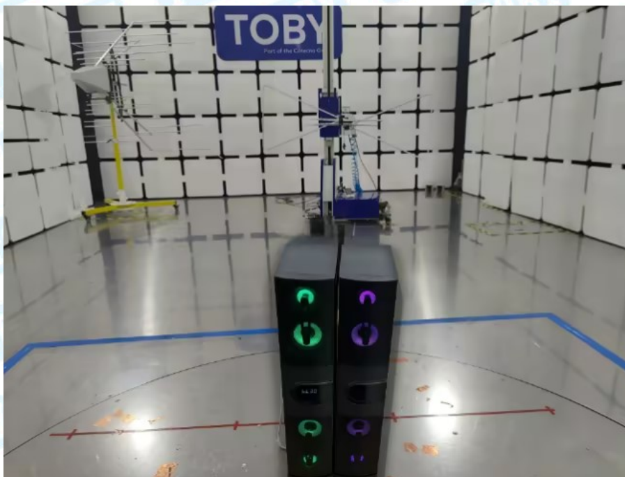
Photo of Setup for Radiated Emission (30MHz~1GHz)
