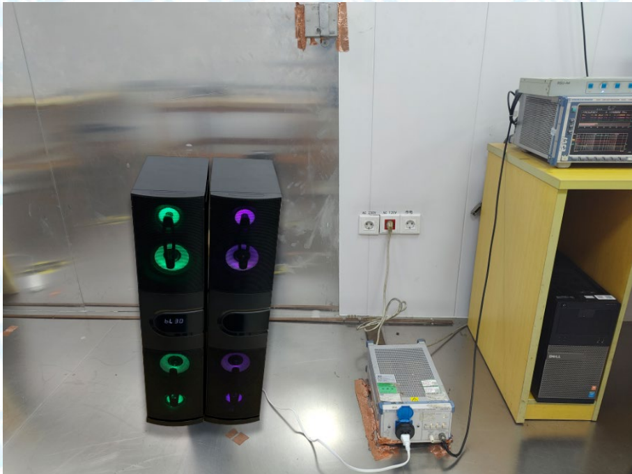
Photo of Setup for Radiated Emission (30MHz~1GHz)
