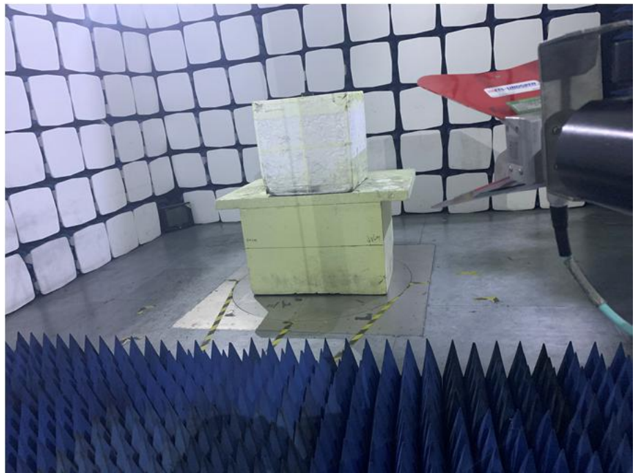
Radiation Emission Test Setup (1GHz to 18GHz)
