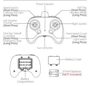
Remove the battery cover on the back of the transmitter, insert three AAA batteries **(not included)** into the battery compartment. Then put the battery cover back to complete the installation.
