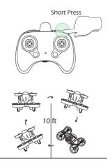
After you get familiar with all the functions of the drone, you can try this amazing flip mode. When the drone is at least 10ft from the ground, press down the () button, then push the right joystick forward/backward or leftward/rightward. The drone will do a flip toward the corresponding direction.
