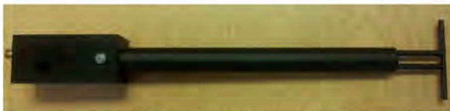
Figure 1 – MVG COMOSAR Validation Dipole
