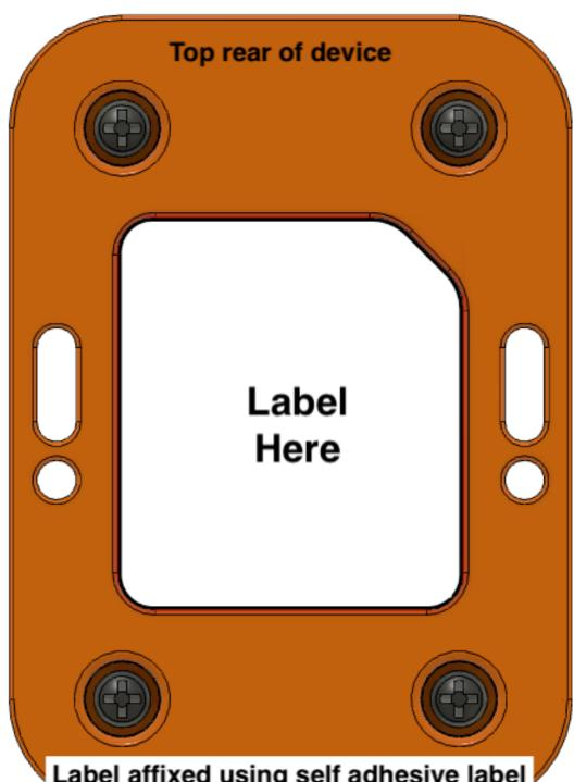
Label affixed using self adhesive label label adhesive is freezer grade and will adhere down to -55 centigrade
