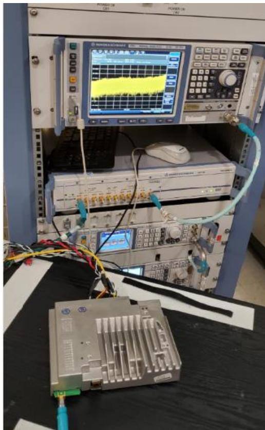
**Figure C2.** Conducted DUT Test setup
