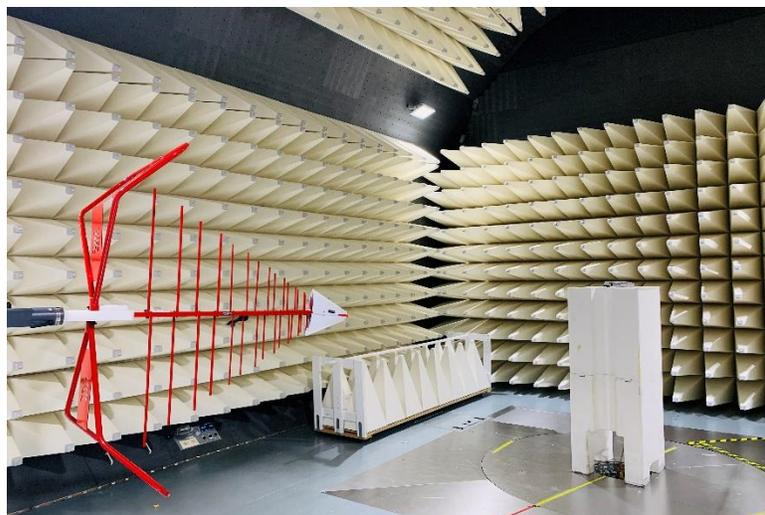
**Figure C4. Radiated Setup**
