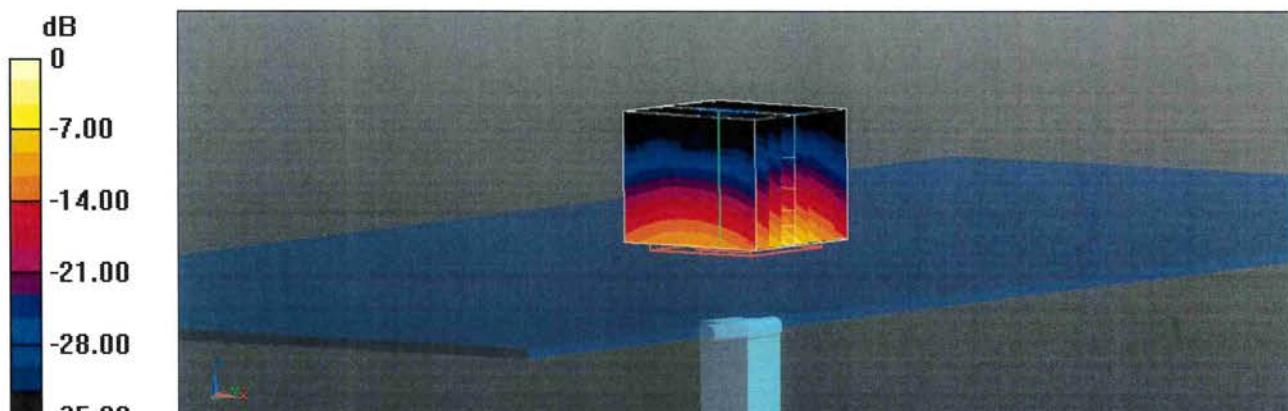
$$0 \text{ dB} = 19.2 \text{ W/kg} = 12.83 \text{ dBW/kg}$$
