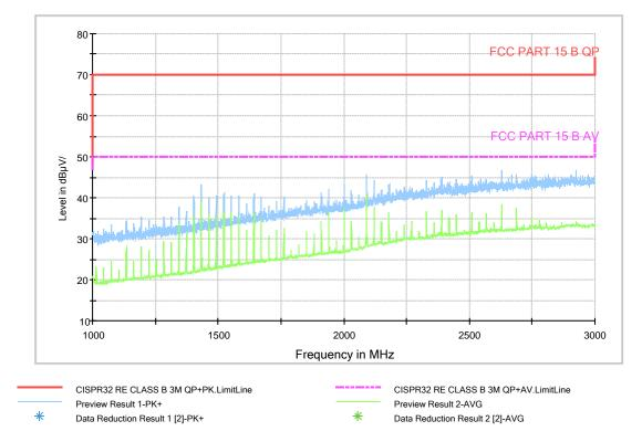
the test results are cumulative (horizontal and vertical)
