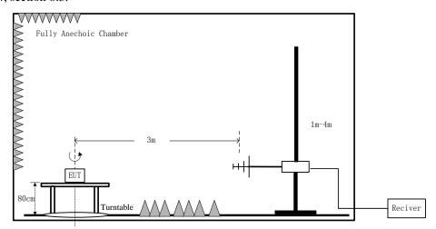
For 1000-18000MHz, the maximal emission value was acquired by adjusting the antenna height, and the table was rotated 360 degree to determine the maximum value of the field strength. Both horizontal and vertical polarizations of the antenna were set during the measurement.
