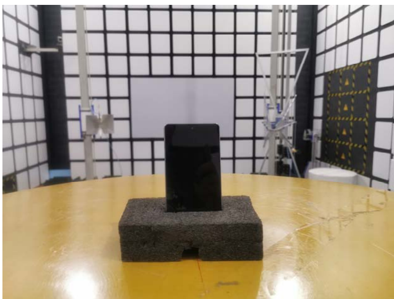
Spurious Radiated Emissions Test setup
