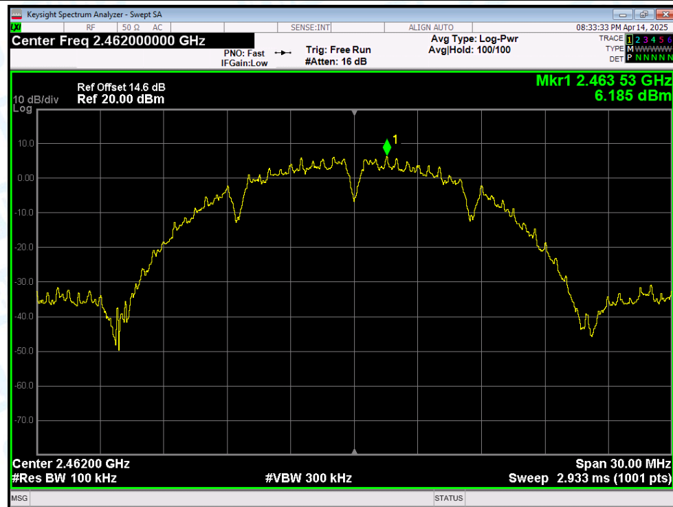
Tx. Spurious NVNT b 2462MHz Ant1 Emission
