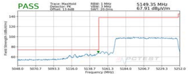
Plot 7-432. Radiated Lower Band Edge Plot MIMO (Peak – UNII Band 1 – 996 Tones)
