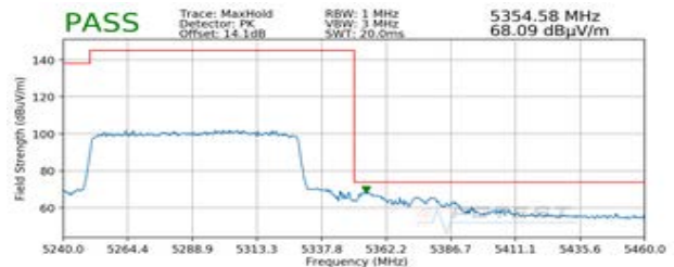
Plot 7-413. Radiated Upper Band Edge Plot SISO ANT2 (Peak – UNII Band 2A – 996 Tones)
