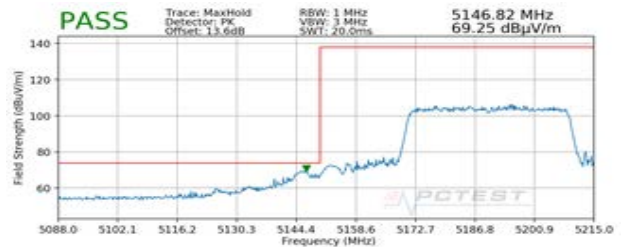
Plot 7-404. Radiated Lower Band Edge Plot SISO ANT2 (Peak – UNII Band 1 – 484 Tones)
