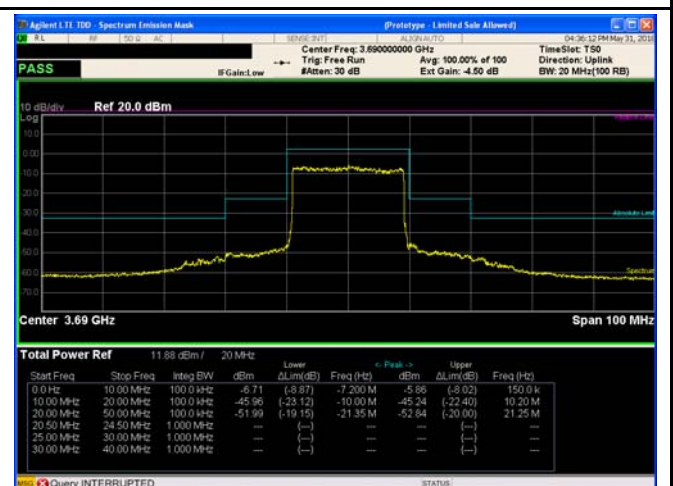
20MHz - Middle CH 16QAM
