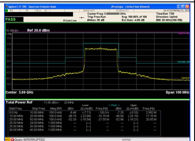
20MHz - Middle CH 16QAM
