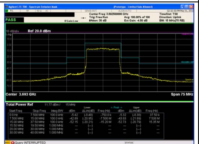
15MHz - Middle CH 16QAM
