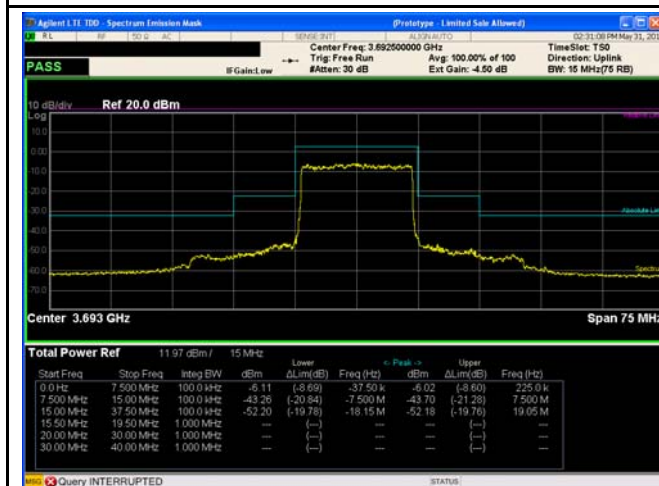
15MHz - Middle CH QPSK
