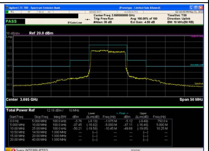
10MHz - Middle CH 16QAM
