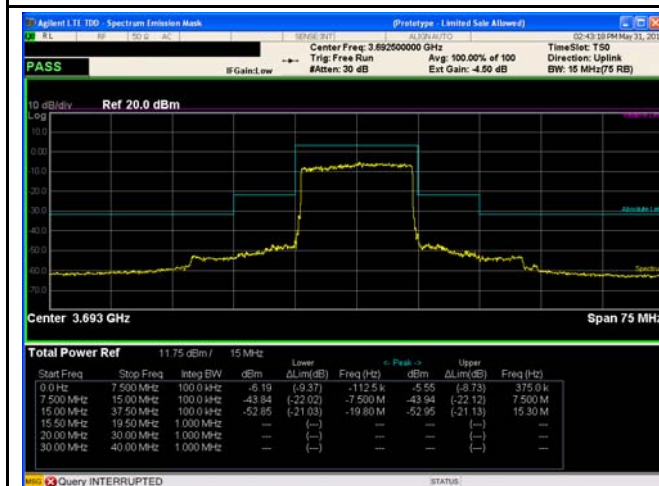
15MHz - Middle CH QPSK
