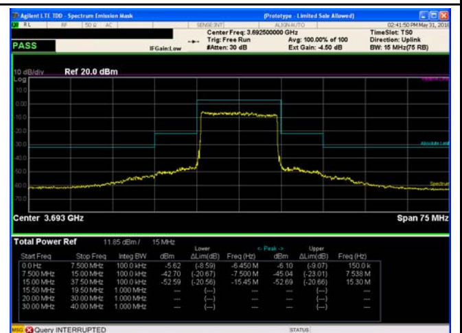
15MHz - Middle CH 16QAM
