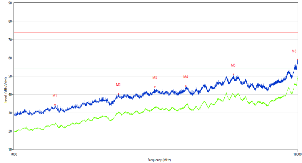
REmission Test case_FCC_Part 15C_FCC 15.247_7GHz-18GHz
