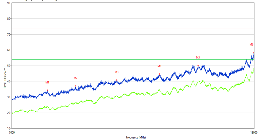
R Emission Test case_FCC_Part 15C_FCC 15.247_7GHz-18GHz
