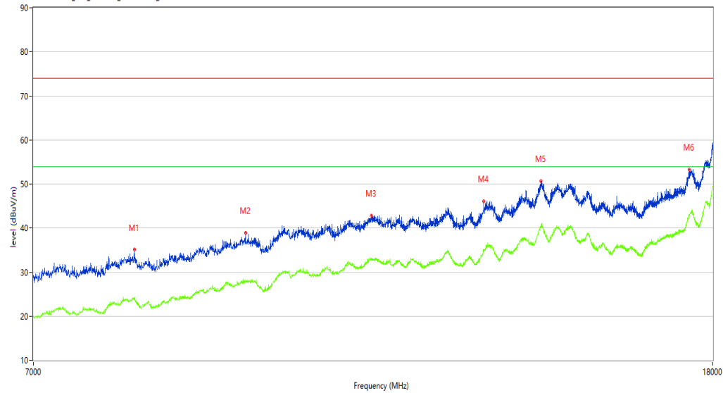
REmission Test case_FCC_Part 15C_FCC 15.247_7GHz-18GHz
