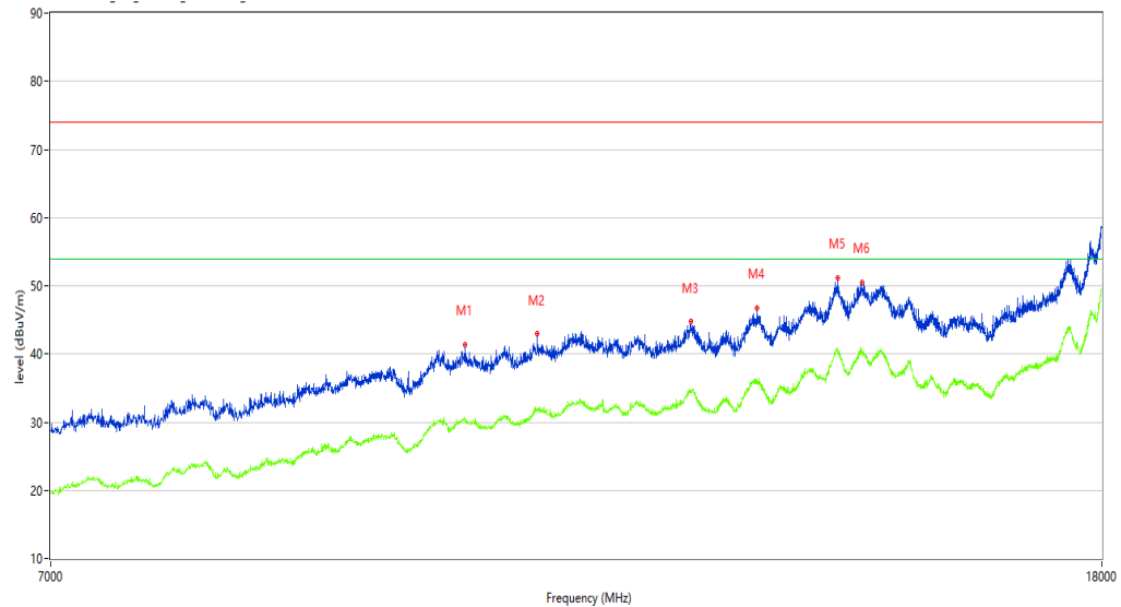
REmission Test case_FCC_Part 15C_FCC 15.247_7GHz-18GHz
