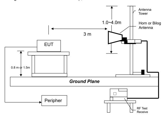
Radiated emission measurements were performed from 9KHz to tenth harmonic or 40GHz.
