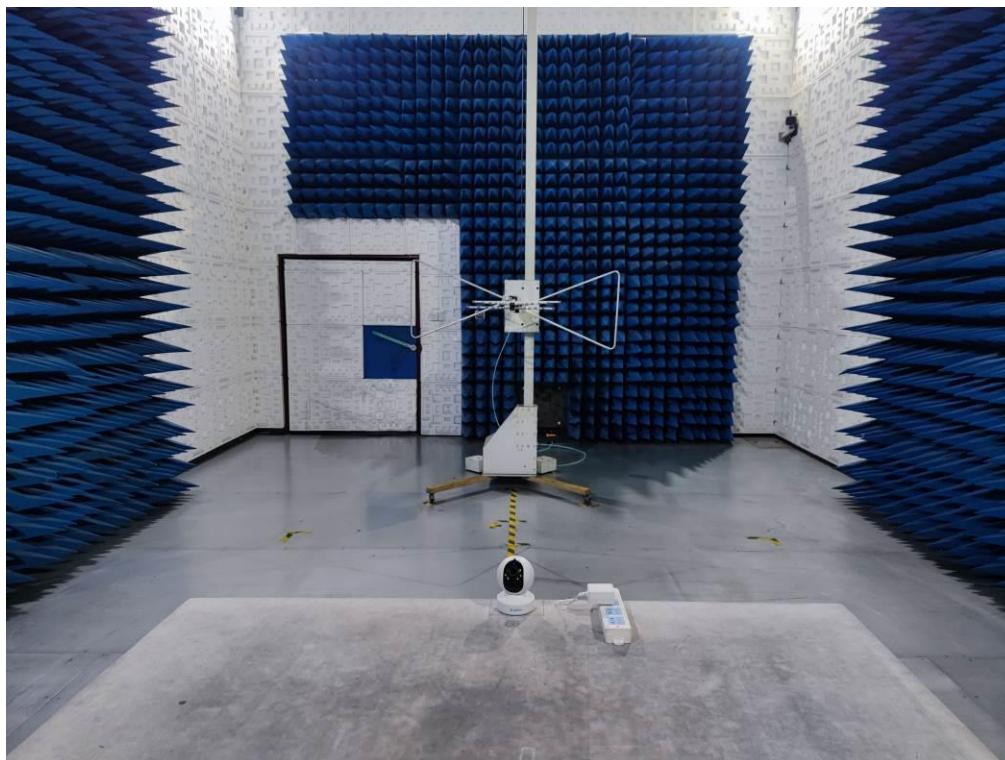
RADIATED EMISSION TEST SETUP ABOVE 1GHz
