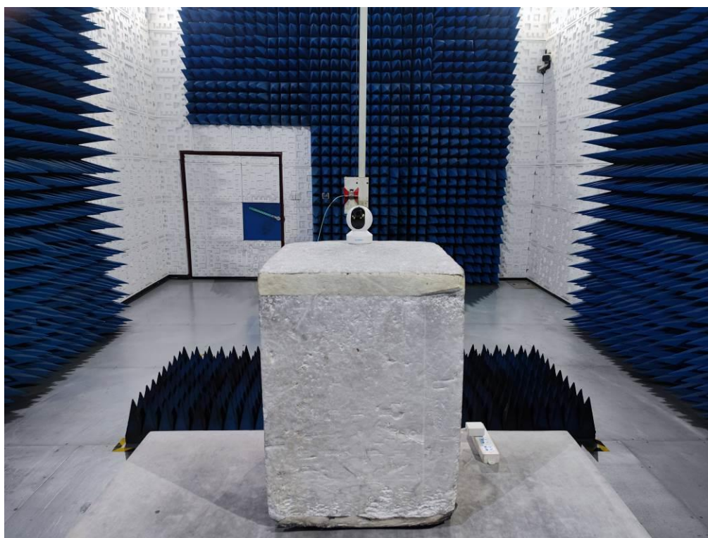
RADIATED EMISSION TEST SETUP ABOVE 1GHz
