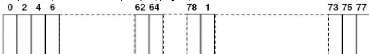
Each frequency used equally on the average by each transmitter. The system receiver has input bandwidths that match the hopping channel bandwidths of their corresponding transmitter and shifts frequencies in synchronization with the transmitted signals.
