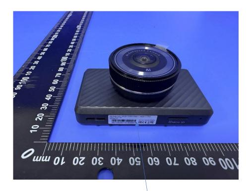
Name: 360 Dash Cam Model: G580H-N560-1 Made in China Input current/voltage: 5V == 1.5A Manufacturer: Botslab Inc.
