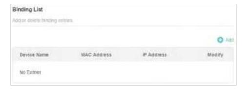
2) Click VIEW CONNECTED DEVICES and select the device you want to bind. Or enter the MAC Address and IP Address that you want to bind.
