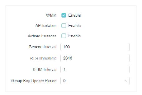
WMM - WMM function can guarantee the packets with high-priority messages being transmitted preferentially.
