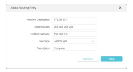
Network Destination: The destination IP address that you want to assign to a static route. This IP address cannot be on the same subnet with the WAN IP or LAN IP of Router A. In the example, the IP address of the company network is the destination IP address, so here enter 172.30.30.1.
