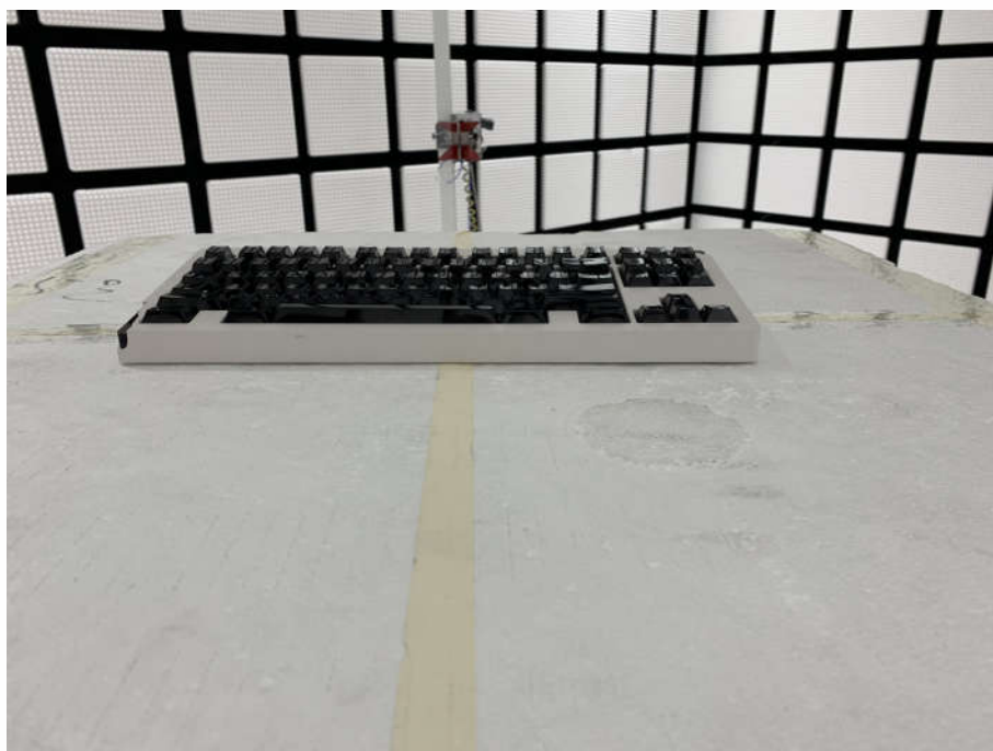
Radiated spurious emission Test Setup-2(Above 1GHz)
