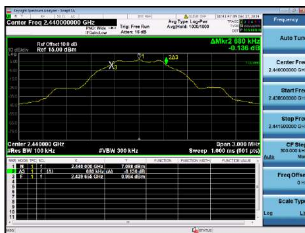
GFSK (BLE 1Mbps) MIDDLE CHANNEL
