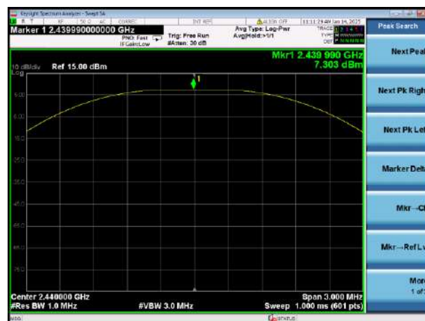
GFSK (BLE 1Mbps) MIDDLE CHANNEL
