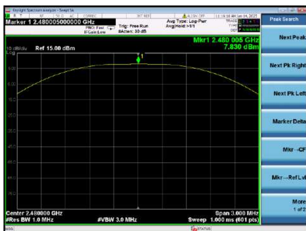
GFSK (BLE 1Mbps) HIGH CHANNEL
