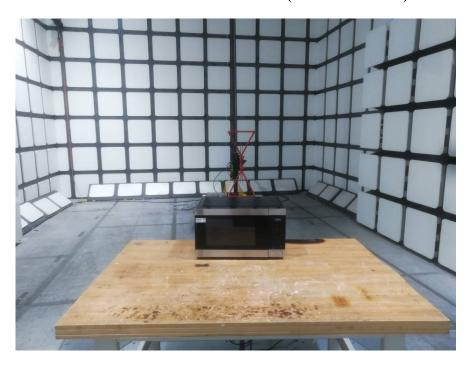
Radiated Emissions - Rear View (30 MHz - 1 GHz)
