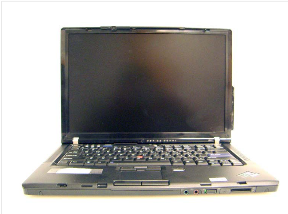
M2 Note (ThinkPad Z61t) - Hybrid CFRP LCD Cover
