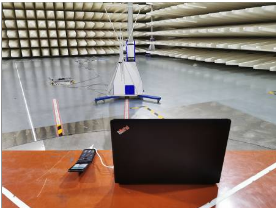
Radiated Emissions Test Setup (with laptop) (30-1000MHz)
