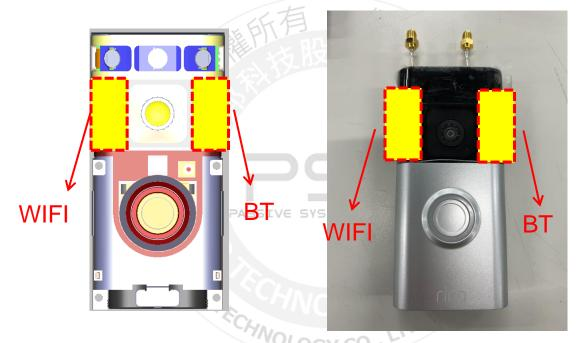
When test WIFI, BT is connected with 50 ohm load.
