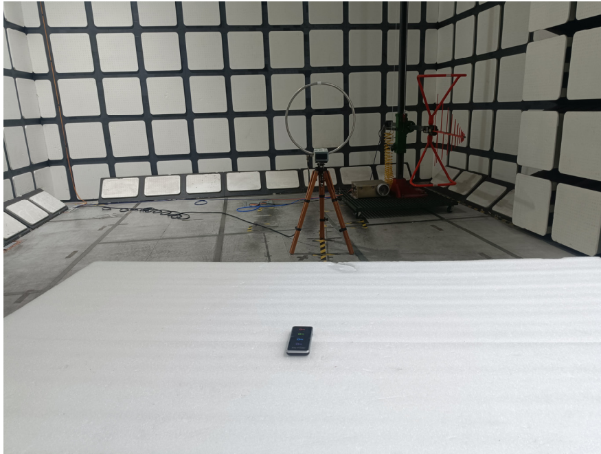
Radiated Emissions View (9 kHz- 30 MHz)
