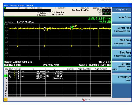
**Duty Cycle** Test Mode: 802.11ac VHT40 & Ch.38
