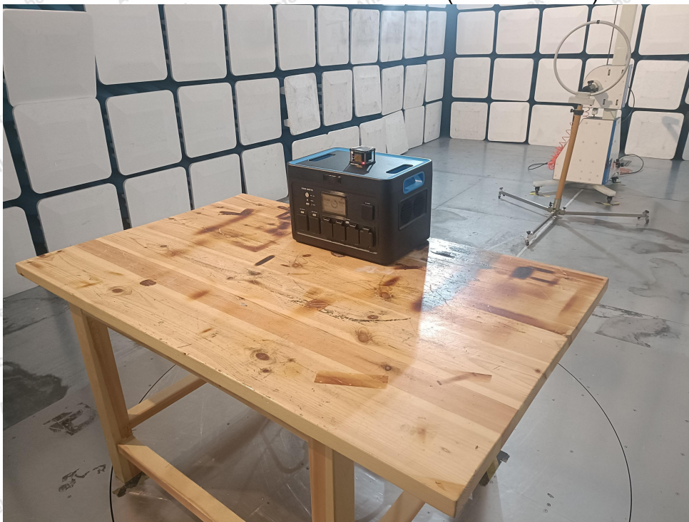
Photo of Radiation Emission Test (below 30MHz)
