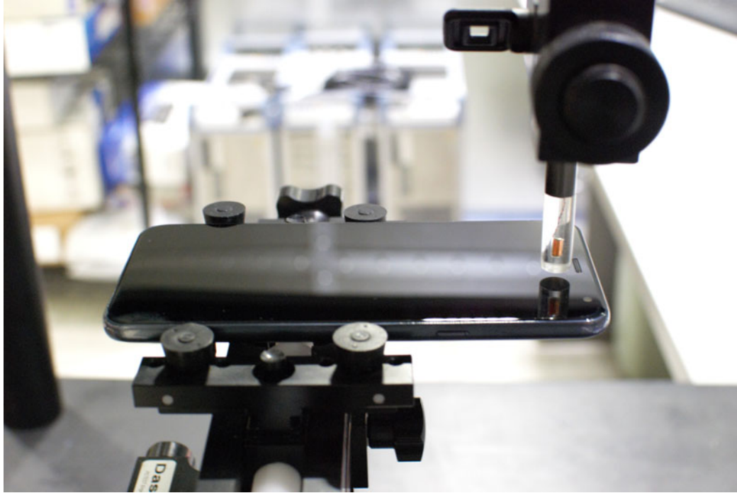
Figure 16-1 Test Setup for Wireless Device
