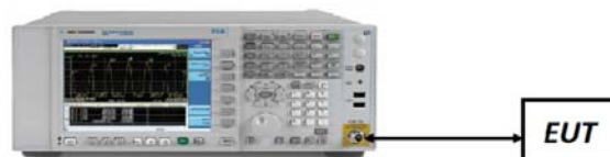
Figure 7-5. Test Instrument & Measurement Setup
