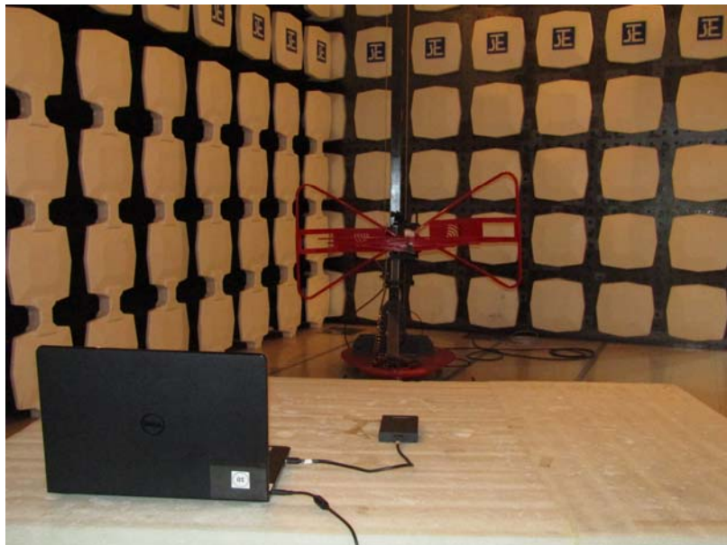
Measurement of Radiated Emission Test Set Up
