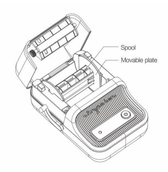
Step4: Load the paper and make the printing side face the print head.
