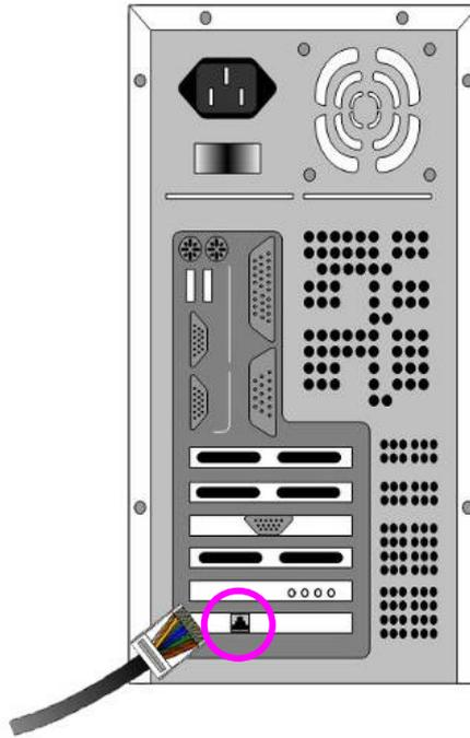
Figure 7 Connecting the SU-200B to the Subscriber's PC
