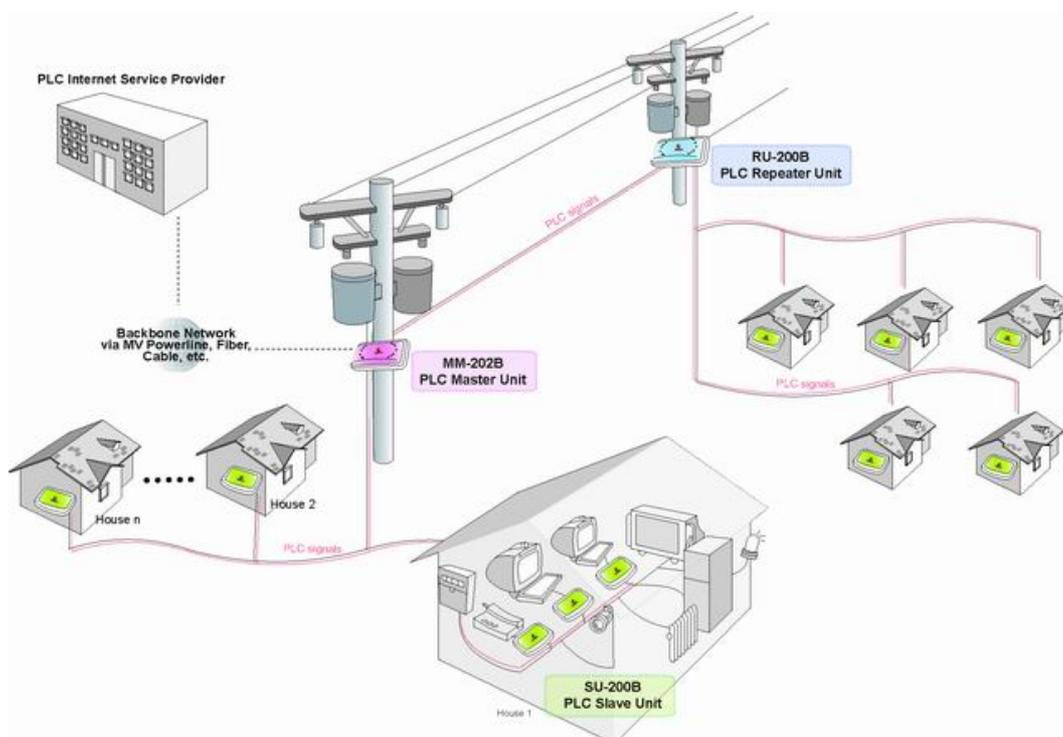
Figure 1 XPAS-200B PLC Internet Access System Configuration
