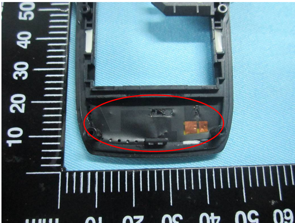
GSM / UMTS - Antenna View
