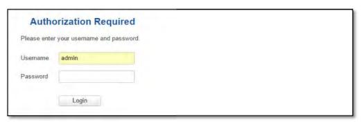
Enter the default password, which is "admin01" into the "Password" field and then either click Login with your mouse or press the Enter key. You have now successfully logged into the RUT955!
