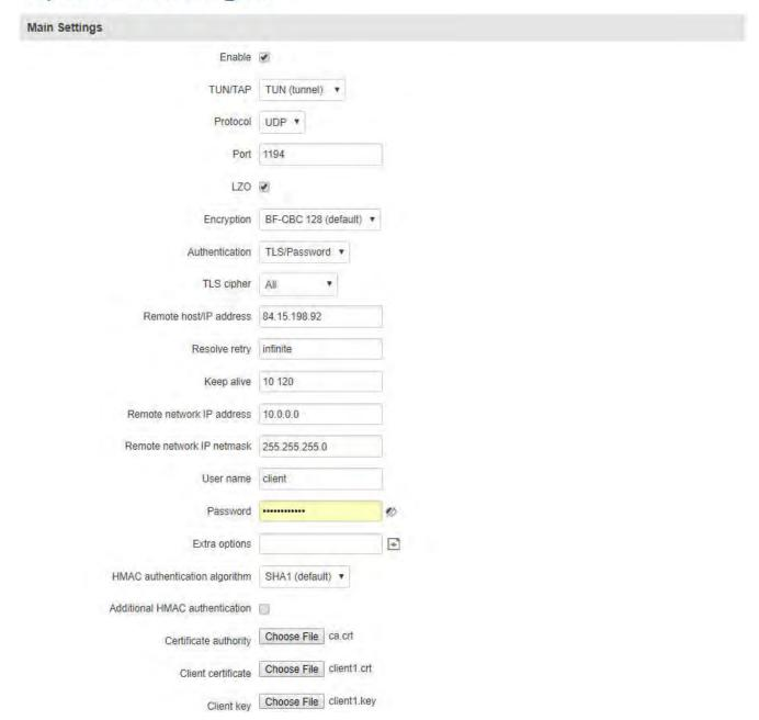
The figure above is a picture of a configured OpenVPN Client instance that uses the UDP protocol and TLS/Password authentication. Comprehensible explanations on how to configure each field are presented in the table below.
