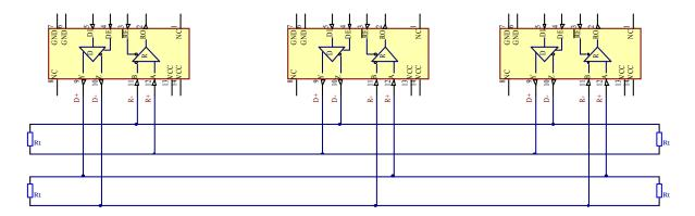
Example 2-wire network electrical connection: to enable a 2-wire RS-485 configuration on a Teltonika router, you need to connect D\_P to R\_P and D\_N to R\_N on the device's RS-485 socket. Termination resistors are placed at each cable end.
