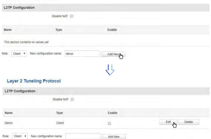
The newly created instance will be disabled and unconfigured. To configure it press the "Edit" button located next to it (as seen in the example above). This action will redirect you to the instance's L2TP Configuration window.
