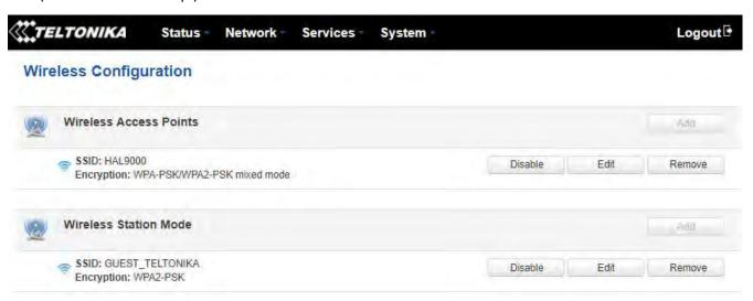
Above is the overview of the Wireless Configuration window. It displays active access points and stations. Here you can disable or enable your Wi-Fi interfaces, remove unwanted access points or stations or enter a configuration window for each Wi-Fi, where you can configure it more thoroughly.
