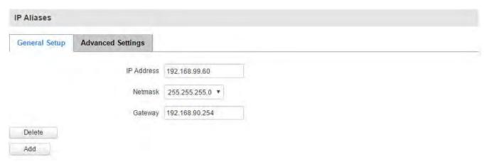
As you can see, the configuration is very similar to the static protocol; only in the example an IP address with a 99th subnet is defined. If some device has an IP in the 99th subnet (e.g., 192.168.99.xxx) and the subnet's gateway metric is "higher" and the device is trying to reach the internet it will reroute it's traffic not to the gateway that is defined in common configurations but through the one that is specified in IP aliases.
