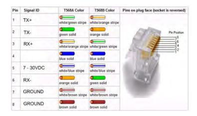
Though the device can be powered over an Ethernet port it is not compliant with the IEEE 802.3af-2003 standard. Powering RUT9xx from a IEEE 802.3af-2003 power supply **will damage the device** as it is not rated for input voltages of the PoE standard.
