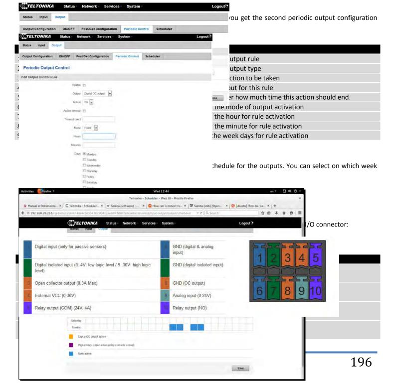
Output (relay) SPST relay output 24V, 4A 1
