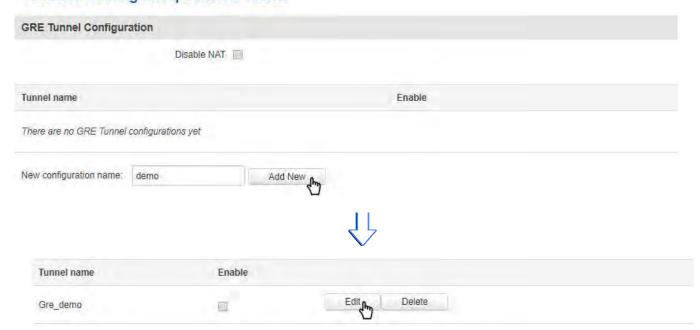
The newly created instance will be disabled and unconfigured. To configure it press the "Edit" button located next to it (as seen in the example above). This action will redirect you to the instance's GRE Tunnel Configuration window.
