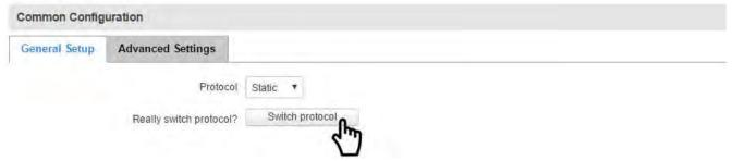
\*The "Switch protocol" button does not apply any changes. In order for the changes to take effect, you must click the "Save" button found at the bottom left corner of the window after you are done making changes.
