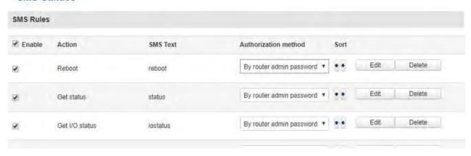
The figure above is an illustration of the SMS Utilities rules list. The entire list contains 26 rules but you are also be provided with the possibility to configure custom ones.
