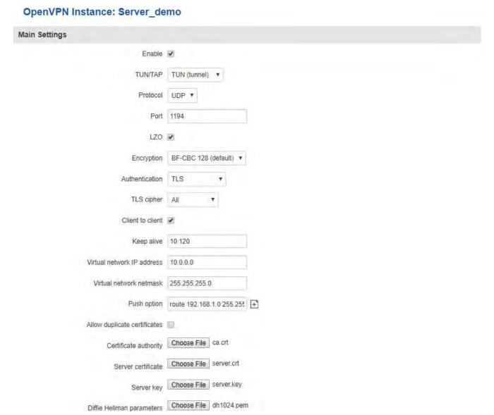
The figure above is a picture of a configured OpenVPN Server instance that uses the UDP protocol and TLS authentication. As you can see, the configuration is similar to OpenVPN Client but with a few key differences. Comprehensible explanations on how to configure each field are presented in the table below.
