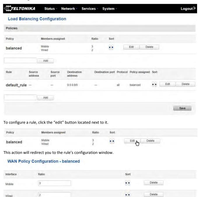
Here you can define the ratio of each WAN interface. In the example above we can see that the mobile interface's ratio is 3, and the wired interface's ratio is 2. This means that  $\frac{3}{5}$  of all traffic will go through the mobile interface, and  $\frac{2}{5}$  will go through the wired interface. After you've finished configuring you Load Balancing rules, go the WAN section and activate Load Balancing for the desired interface.
