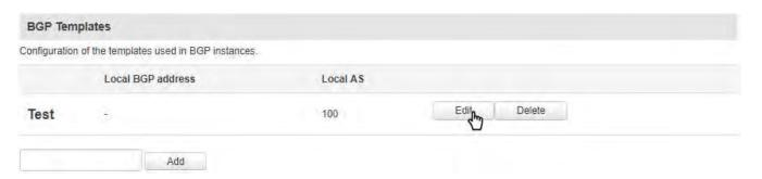
After this you will be redirecting to the BGP protocol's configuration window where you can configure your new BGP protocol in detail.
