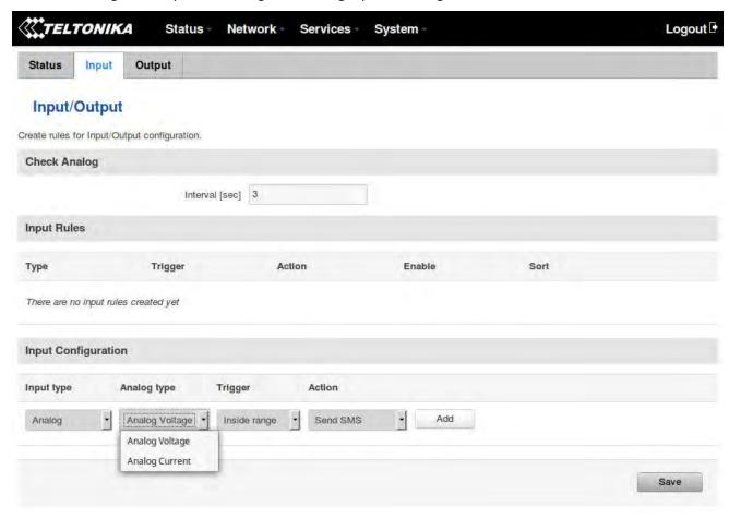
In the input rules section you can create and modify the rules for action after specific input triggering.
