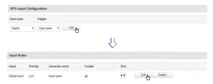
This will create a new unconfigured Input rule. To configure it press the **Edit** button located next to the newly created rule.
