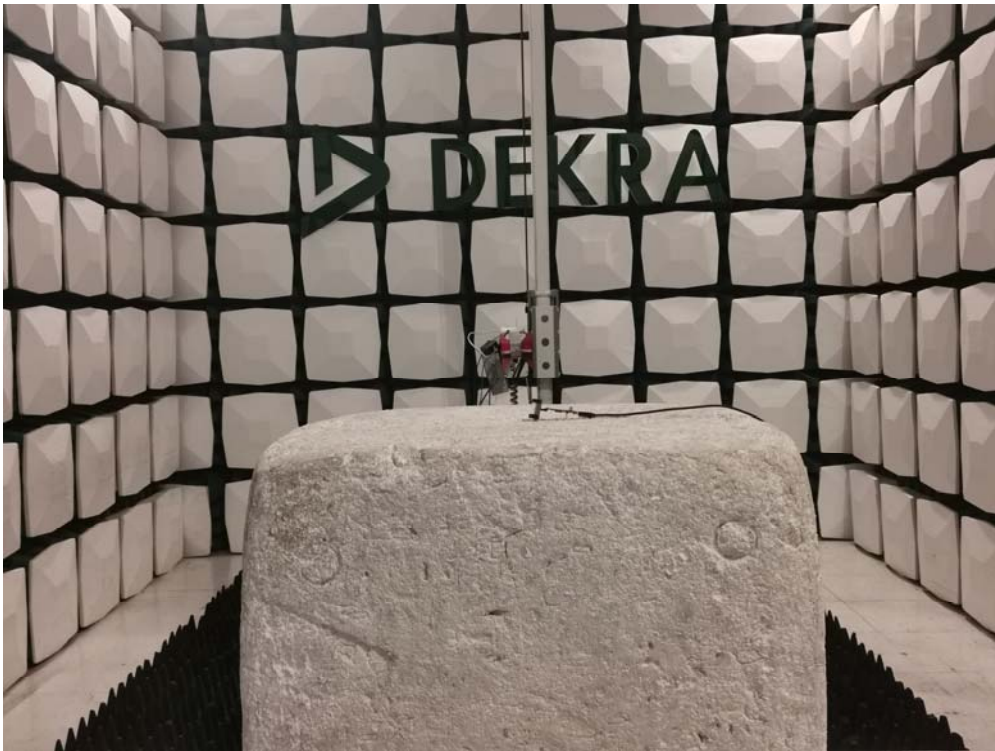
Description: Radiated Emission Test Setup for 1~18GHz
