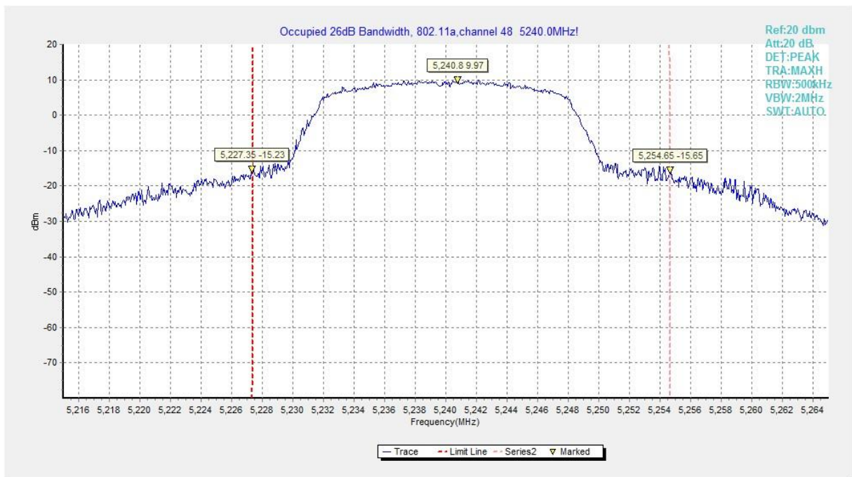
Fig.3 Occupied 26dB Bandwidth (802.11a, 5240MHz)
