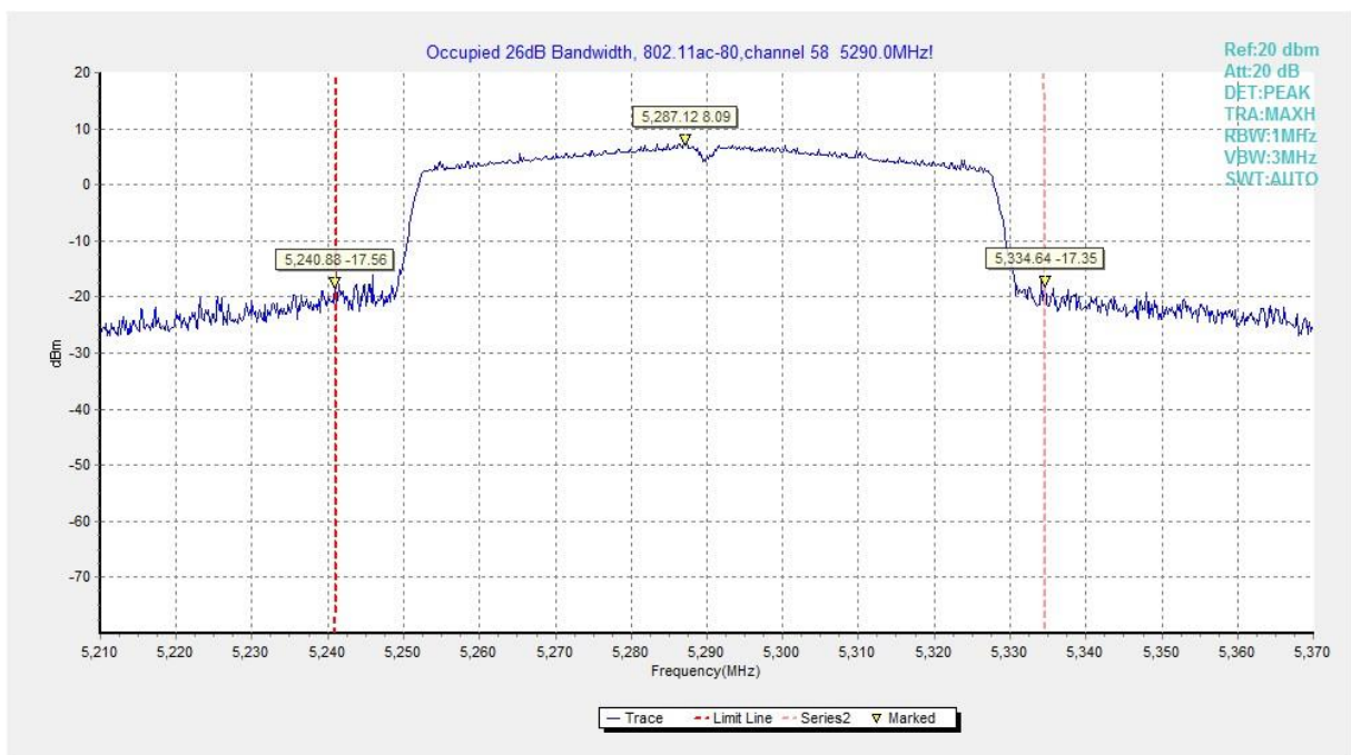
Fig.27 Occupied 26dB Bandwidth (802. 11ac-HT80, 5290MHz)
