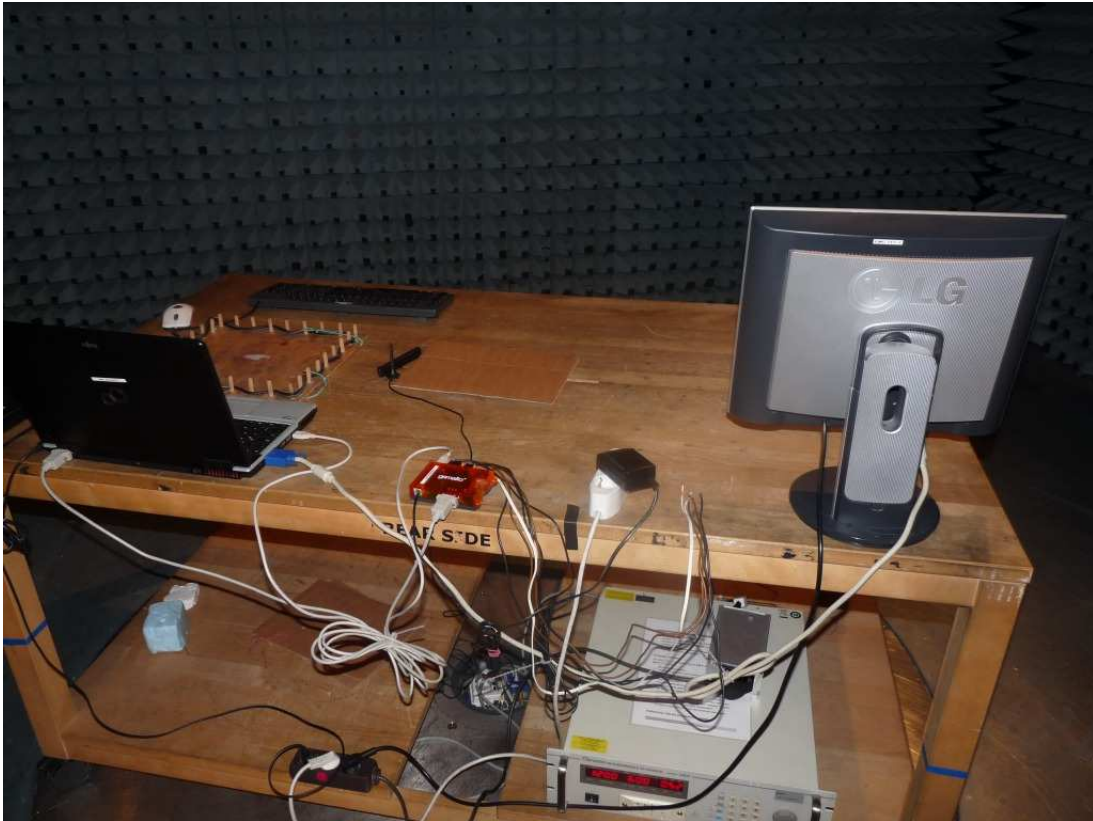
Photo 2: Test setup AA01 for radiated measurements, unintentional radiator §15) single device setup, computer peripheral.
