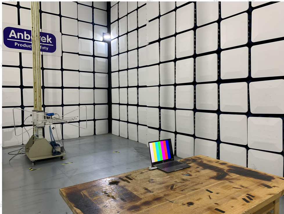
Photo of Radiation Emission Test
