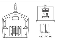
Take out the battery cover from the back of remote control,and install 4 batteries(size AA) into the battery case correctly (Refer to the picture), then shut the battery cover.
