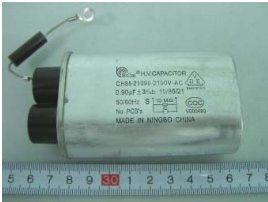
EUT – Capacitor View
