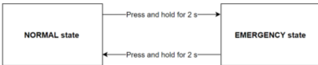
Figure 3-3: EB activation and deactivation block diagram
