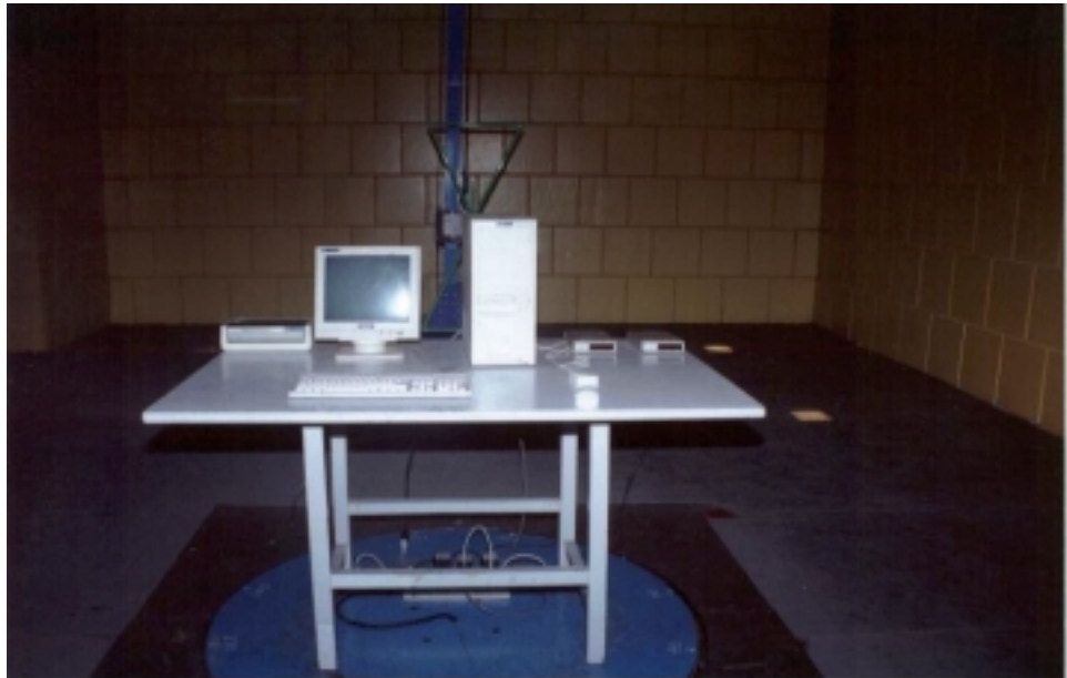
FRONT VIEW OF RADIATED MEASUREMENT
