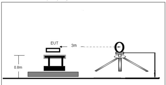
(B) Radiated Emission Test-Up Frequency 30MHz~1GHz
