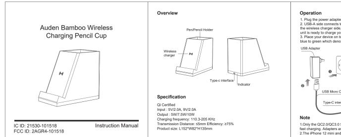
Plug the power adapter into the wall socket (adapter not included)
