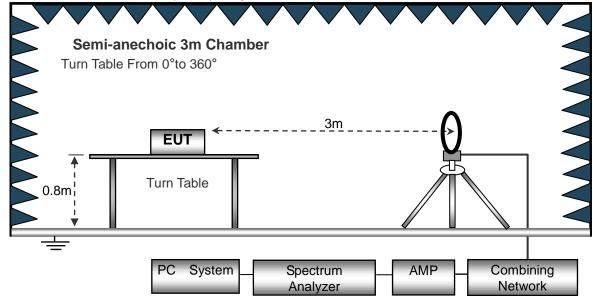
(B) Radiated Emission Test-Up Frequency 30MHz~1GHz
