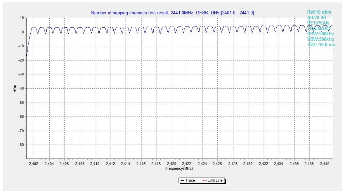
Fig.94. Number of hopping frequencies: GFSK, Channel 0 - 39
