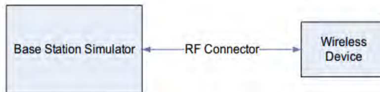
Figure 10.2 Power Measurement Setup
