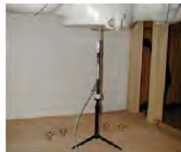
Figure 11.1 Dipole Verification Test Setup Diagram & Photo
