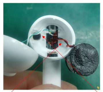
Control the battery wire length of the left ear to 25mm, wrap the battery wire with 4-5 turns, and place the battery pole ear upward
